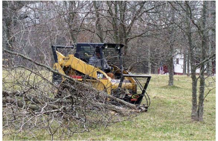
This machine, equipped with a shear (hydraulic scissors) was used to remove about 140 Honey Locust from the County Farm.
